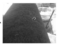
**STEP 3:** Place the supplied socket cup set screw into the enclosure, leaving 1/4" exposed.
